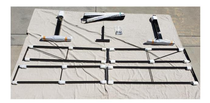
Step 2: Assemble the Truss Net sections (With slant brace bar) to the end posts
