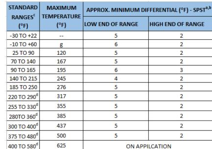
A differential is the difference between the opening and closing (make/break) points of the switch contacts. **Differentials** are approximately 50% wider for SP-DT and DP-ST 1 NO & 1 NC circuitry. For capillary tubing over 10 ft. in length, the minimum differential is 1-1/2 times that shown. Differential capabilities of nonstandard bellows will be provided on application.
