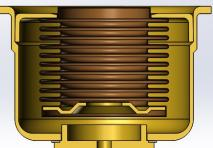
Seamless phosphor bronze bellows construction in all models provides a long life and accurate repeatability at set point. Optional metals available.
