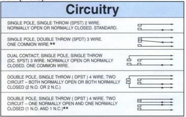
\*\*NOTE: Manual Reset Circuit Option May Shock Open. Field adjustable differential optional on SPST only. Minimum differential is approximately 1-1/2 times the SPST minimum differential.
