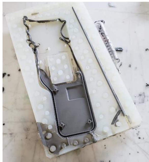
Pic right: failed part for an AcuShot housing in a silicone mold.
