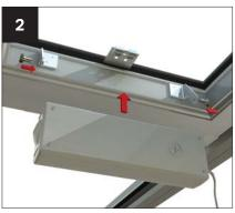
Offer up the motor to the brackets on vent Screw motor pin into the top edge of the body and secure.
