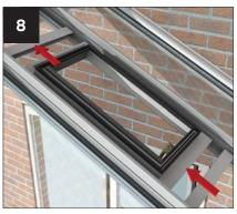
edge of vent body and then slide vent body into upper H section. Repeat process for lower glazing panel. H section and insert along top and bottom edges of both H into trailing edge of vent body. Ensure glazing/vent body are central between the two glazing bars.
