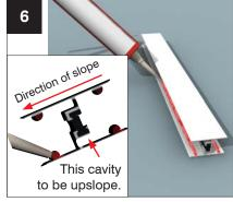
Now is the time to glaze the vent body into the roof. The vent is glazed in using two H sections at top and bottom. Prepare the upper H section using appropriate sealant in the four positions shown.
