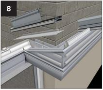
Following steps for the installation of box Place the short lengths of firring top cap and modified starter bar on to the two bolts. Please note that the bolts should be staggered, one each side of the bar.
