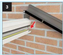
Fit the pre formed soaker trim to each starter bar, tighten the bars at the ridge and then at the eaves. Ensure the bar caps have been fitted.
