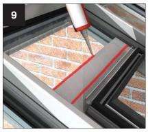
Now is the time to glaze the vent body into Apply bead of appropriate sealant to top Using appropriate sealant (low modulus neutral cure for polycarbonate and MS Polymer for self cleaning glass), run beads sections.
