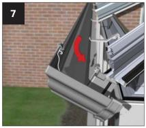
Locate the back edge of each section gutter into the slot in the gutter bracket.
