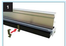
Attach spring clips (LAN014) to side of glazing bar - to each side of bar - 50mm from top of transom bar - 100 mm from Spring clips in position. eaves (both hip and transom). Push the leg in under the gasket and spring around the underside as shown. Ensure the clips are fully pushed on.
