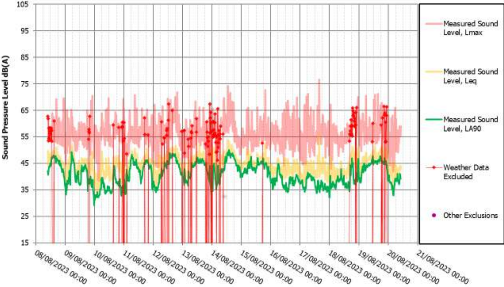
Figure B4 Results of the Noise Monitoring at the south end of the Site)– Noise Levels L_{Aeq} , L_{A90} , L_{max} , 15mins
