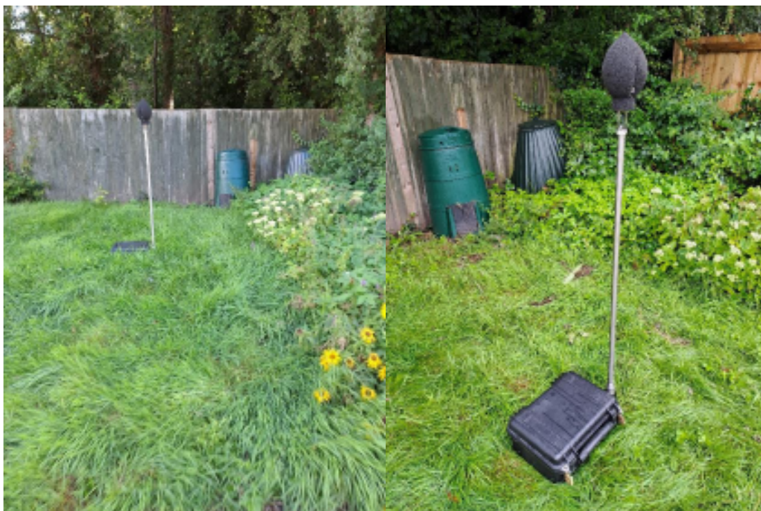
Figure B14 Noise Monitoring Setup at 2 Nantymor Cottages
