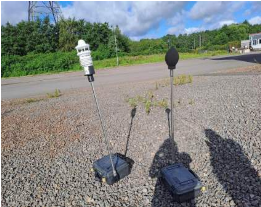
Figure B3: Noise Monitoring Setup at the south end of the Site
