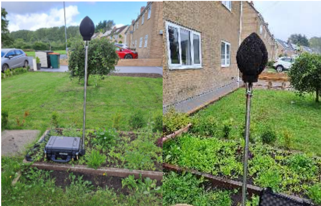
Figure B1 Noise Monitoring Setup at 10 Church Crescent
