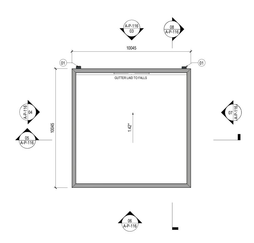
02 SUBSTATION ROOF PLAN SCALE: 1:100
