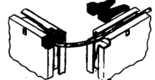
Plastic cable retainers inserted and removed.
