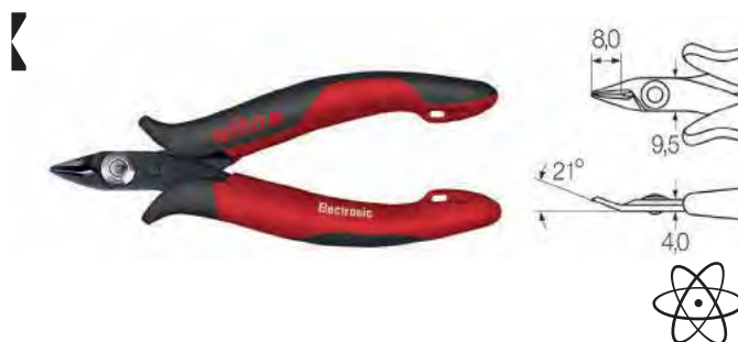
very narrow, pointed head without bevelled edge
