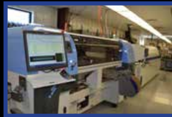
Surface mount placement equipment (SMT) meeting all the newest board and component designs
