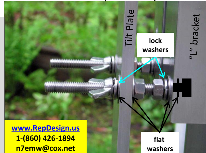
(c) Tilt Plate 4 longer bolts attach it to L brackets)
