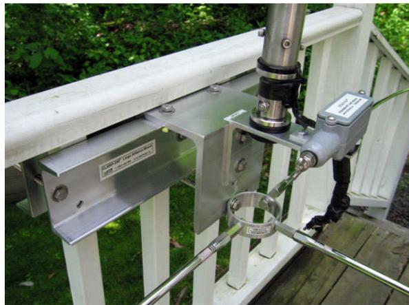
Photo of AMB-BKT-1 bolted to a **BKT-NissanTrac-1** "slide-in" mount for Nissan pickups. Then antenna is a High Sierra "Sidekick" with "long quick disconnect".
