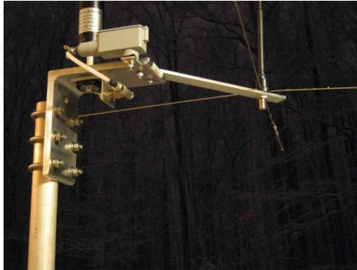
2. Photos of **CLAMP-150** “clamp to anything” mount. The left and right photos show a High Sierra Sidekick HF screwdriver antenna with a 2m-70cm multi band antenna. The middle photo shows a Buddipole™ dipole in “L” configuration with a 2m-70cm antenna.
