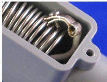
**Figure 5:** View of rubber pad under coil, to access the mounting plate bolt head. Not visible is the new solder lug (Revision 2) that is under the rubber pad and soldered to the ground side of the coil.
