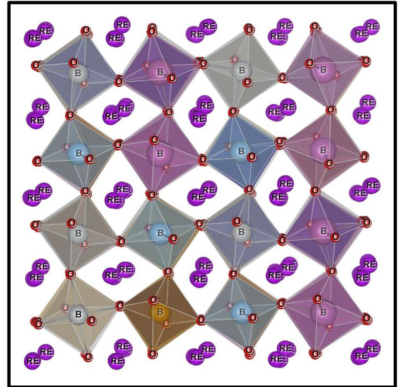
Figure 2: The synthesized CCOs are a variation of  $\text{A}^{2/3}\text{B}^{3/4}\text{O}_3^{2-}$  structure with rare earth metals at the A site and various elements at the B site.
