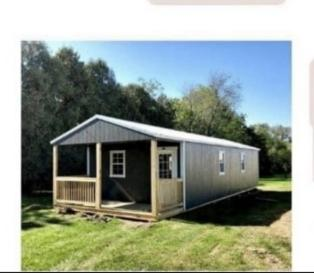
OUR BUILDINGS ARE DESIGNED TO REST DIRECTLY ON THEIR SKIDS. IN ORDER TO LEVEL THE BUILDING WE USE TREATED WOOD BLOCKS. IF YOU WOULD LIKE TO HAVE YOUR BUILDING ON CONCRETE BLOCKS, WE ONLY REQUIRE THAT YOU PROVIDE THE BLOCKS.
