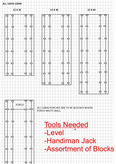
Properly blocked and level buildings increase customer satisfaction by ensuring windows and doors open and close, and help prevent leakage.
