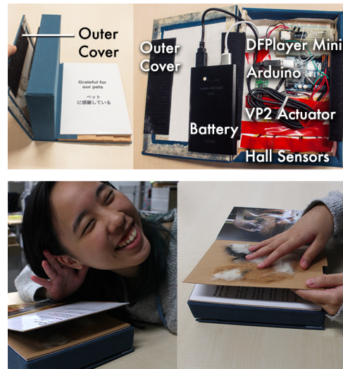
Fig. 1. [Top] Hardware set up of our book prototypes. [Bottom] Users can listen to the storyteller share their story on one set of pages. Then experience the story through passive and active haptic sensations.
