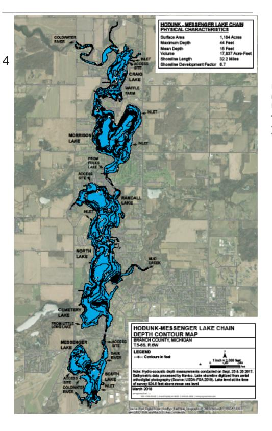
High-definition hydro-acoustic mapping of the Hondunk-Messenger Lake Chain was conducted in 2017 by Progresseve AE and processed data was used to create bathymetric mapping.
