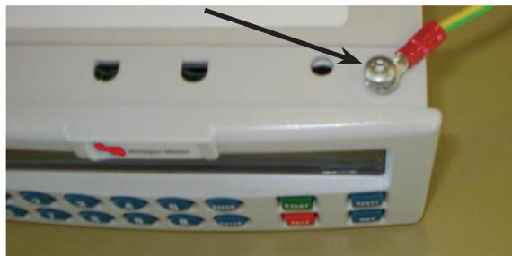
Figure 3: Grounding location, top view
