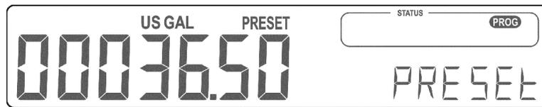
Figure 19: Example display information during programming preset value
