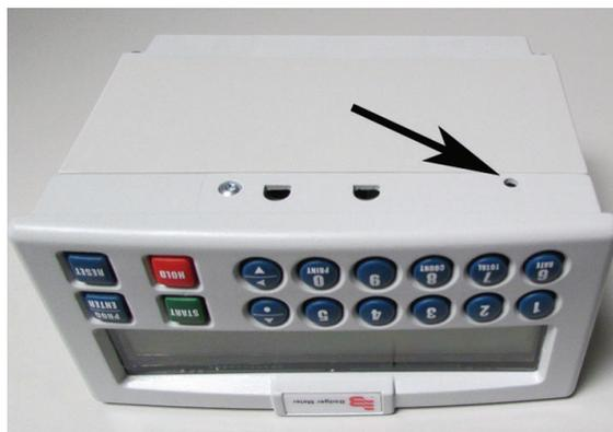
Figure 4: Grounding location, bottom view
