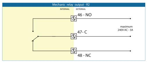
Figure 17: Mechanical relay output R2
