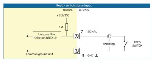
Figure 7: Reed switch signal input
