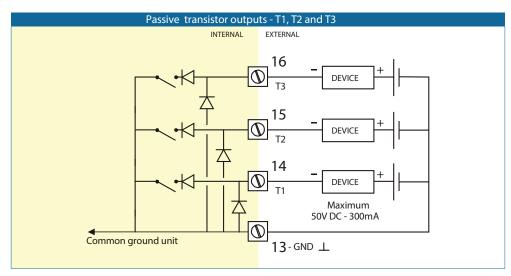
Figure 14: Passive transistor outputs T1, T2 and T3
