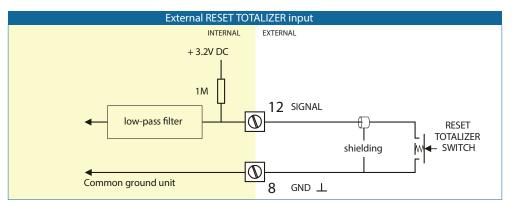
Figure 13: External reset totalizer input
