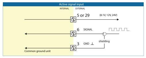
Figure 9: Active signal input
