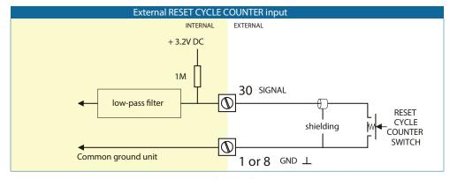
Figure 15: External reset cycle counter input
