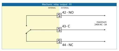
Figure 16: Mechanical relay output R1
