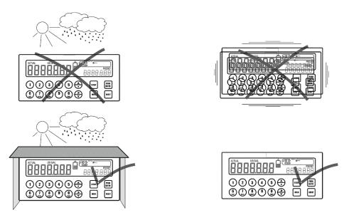
Figure 1: Acceptable installation conditions
