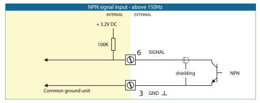
Figure 8: NPN signal input
