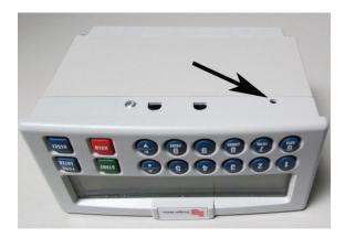
Figure 4: Grounding location, bottom view
