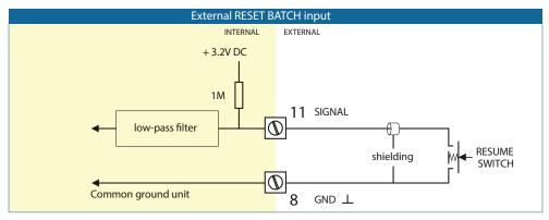
Figure 12: External reset batch input
