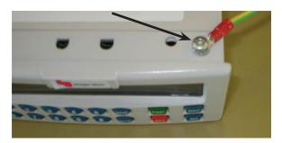
Figure 3: Grounding location, top view
