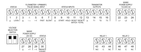
Figure 6: Overview of terminal connectors
