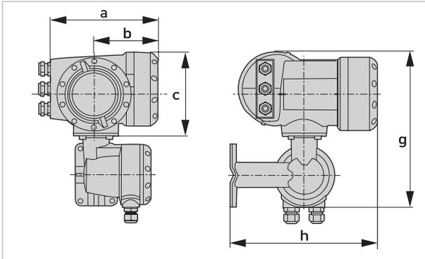
Figure 8-1: Dimensions for field housing (F) - remote version
