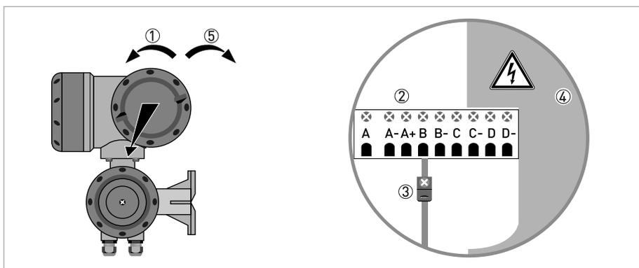
Figure 4-4: Terminal compartment for inputs and outputs in field housing
