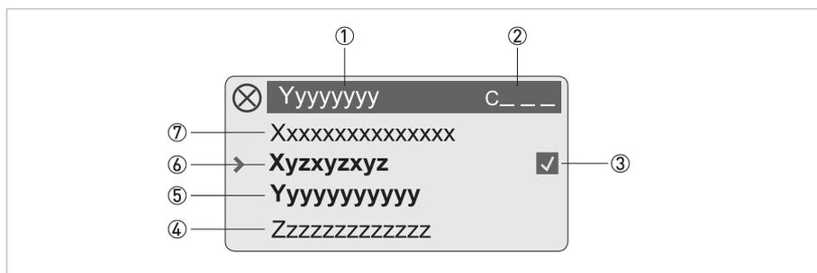
Figure 6-5: Display when previewing parameters, 4 lines
