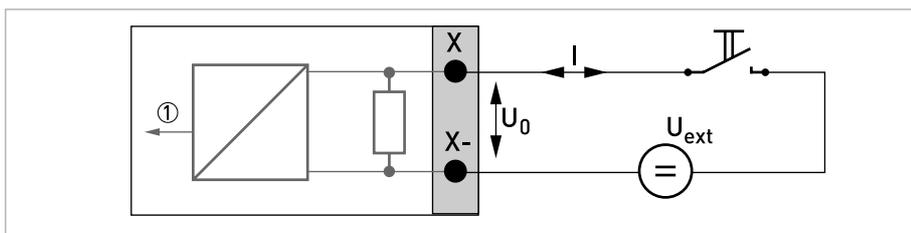
Figure 4-26: Control input passive  $C_p$  Ex i
