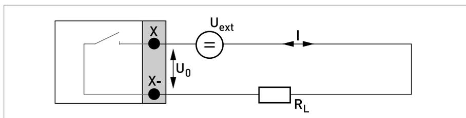
Figure 4-9: Status output / limit switch passive  $S_p$ **Control input passive, basic I/Os**
