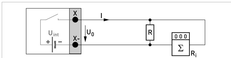
Figure 4-13: Pulse / frequency output active  $P_a$
