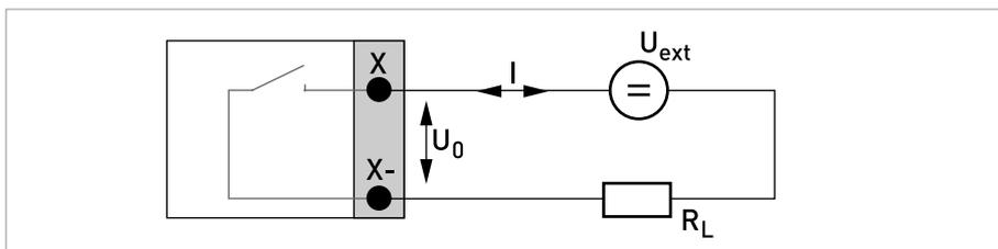
Figure 4-17: Status output / limit switch passive  $S_p$
