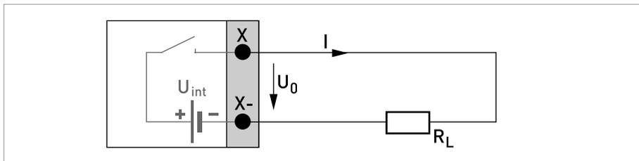
Figure 4-16: Status output / limit switch active  $S_a$
