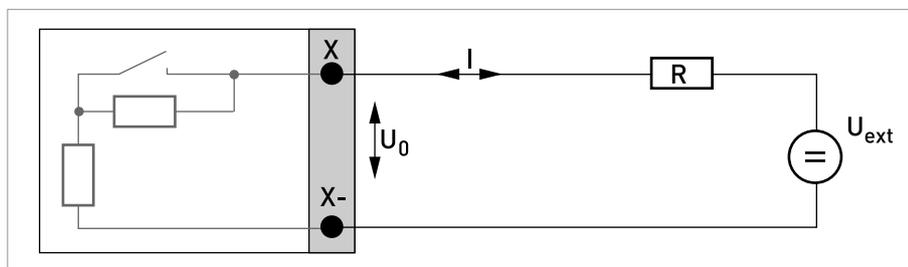
Figure 4-15: Pulse and frequency output passive  $P_N$  acc. to NAMUR EN 60947-5-6
