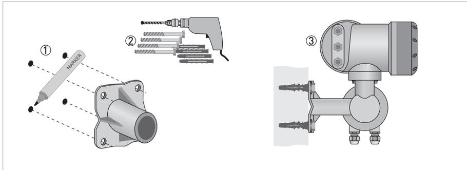
Figure 3-2: Wall mounting of the field housing
