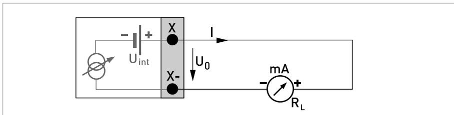
Figure 4-22: Current output active  $I_a$  Ex i
