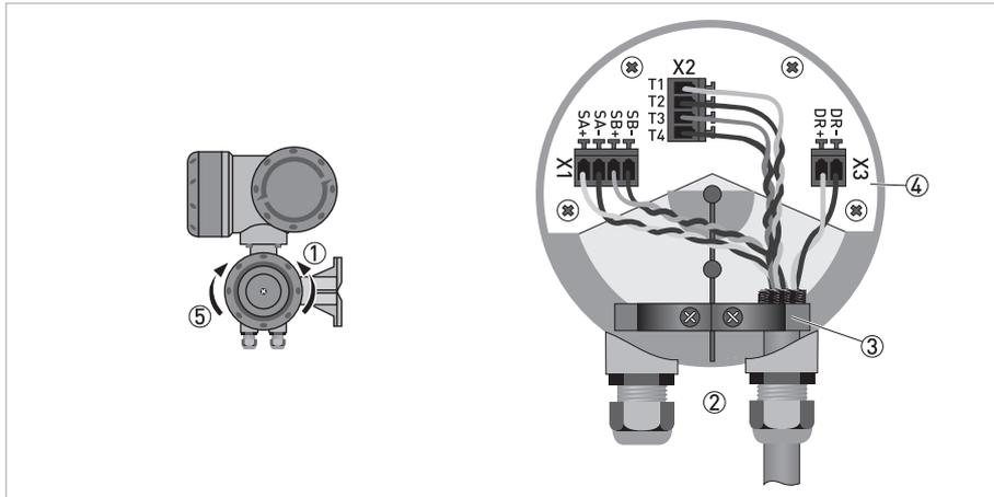
Figure 4-1: Connection of signal cable - Field housing and connection box for sensor
