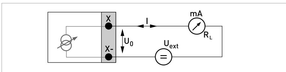
Figure 4-23: Current output passive  $I_p$  Ex i
