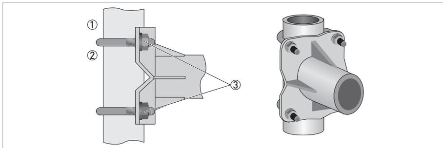
Figure 3-1: Pipe mounting of the field housing
