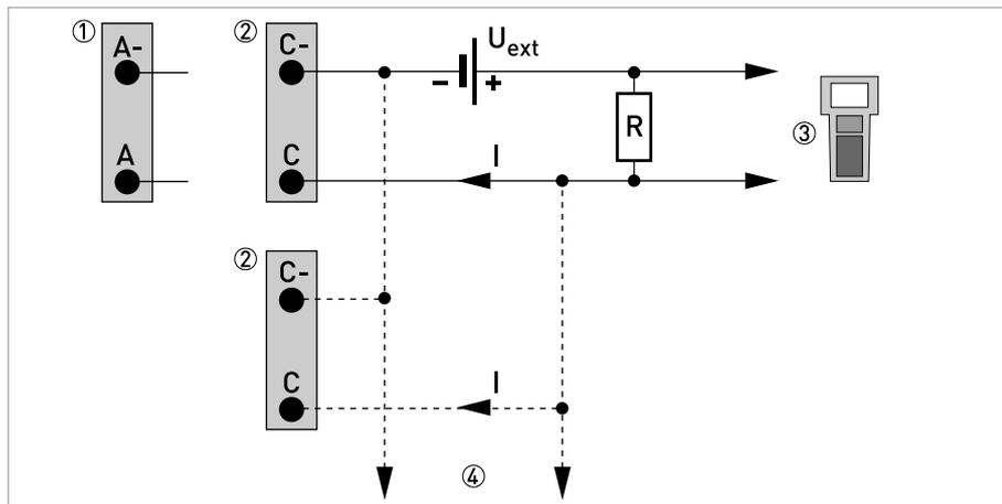
Figure 4-28: HART<sup>®</sup> connection passive ( $I_p$ )
