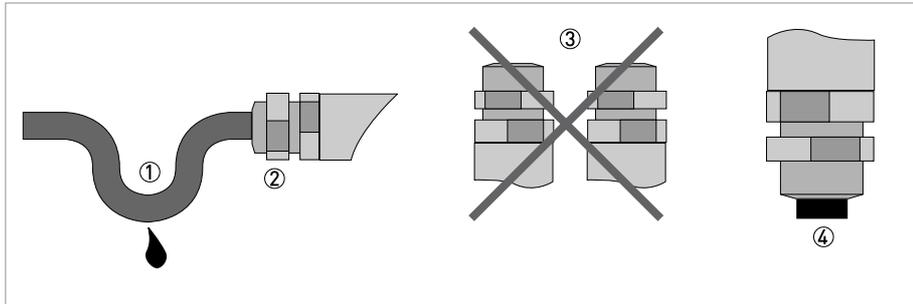
Figure 4-5: Protect housing from dust and water
