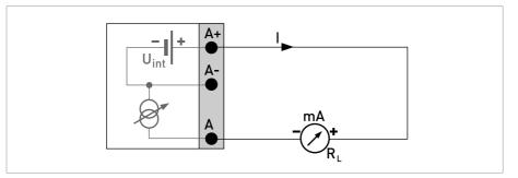
Figure 4-6: Current output active I<sub>a</sub>
