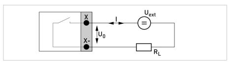
Figure 4-17: Status output / limit switch passive Sp
