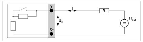
Figure 4-18: Status output / limit switch S<sub>N</sub> acc. to NAMUR EN 60947-5-6
