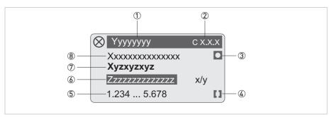
Figure 6-4: Display when setting parameters, 4 lines
