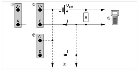
Figure 4-28: HART<sup>®</sup> connection passive (I<sub>p</sub>)
