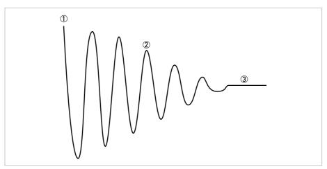
Figure 6-8: Vibration behaviour during pressure suppression
