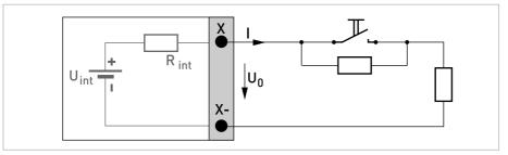
Figure 4-21: Control input active C<sub>N</sub> acc. to NAMUR EN 60947-5-6
