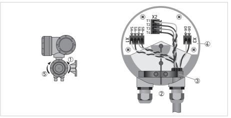
Figure 4-1: Connection of signal cable - Field housing and connection box for sensor
