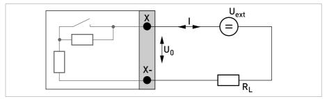
Figure 4-25: Status output / limit switch  $\rm S_N$  acc. to NAMUR EN 60947-5-6 Ex i
