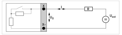
Figure 4-15: Pulse and frequency output passive  $\mathsf{P}_{\mathsf{N}}$  acc. to NAMUR EN 60947-5-6
