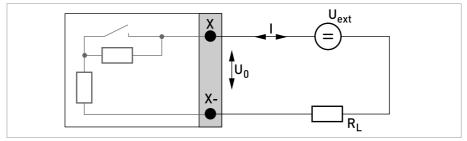
Figure 4-24: Pulse/frequency output passive P<sub>N</sub> acc. to NAMUR EN 60947-5-6 Ex i
