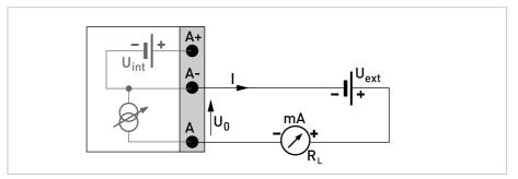
Figure 4-7: Current output passive Ip
