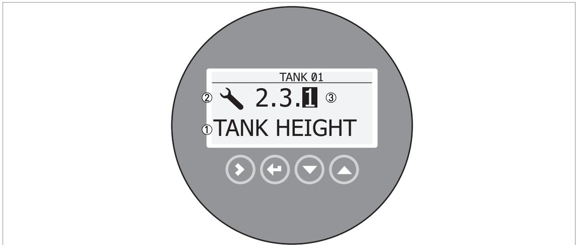
Figure 5-2: Local display screen layout in configuration mode
