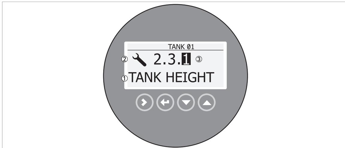
Figure 6-1: Local display screen layout in configuration mode
