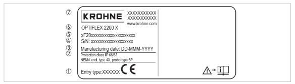
Figure 2-5: Remote (F) version: Non-Ex nameplate attached to the probe assembly
