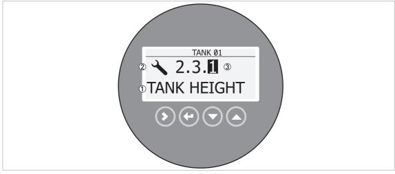
Figure 6-1: Local display screen layout in configuration mode
