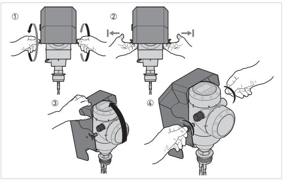
Figure 3-43: How to open the weather protection
