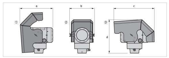
Figure 8-13: Weather protection option for Compact / Horizontal and Remote versions
