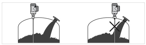
Figure 3-21: Do not install the probe near to a product inlet
