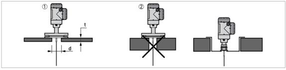
Figure 3-10: Installation on a concrete roof
