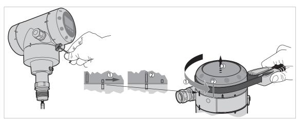
Figure 4-2: How to open the terminal compartment cover
