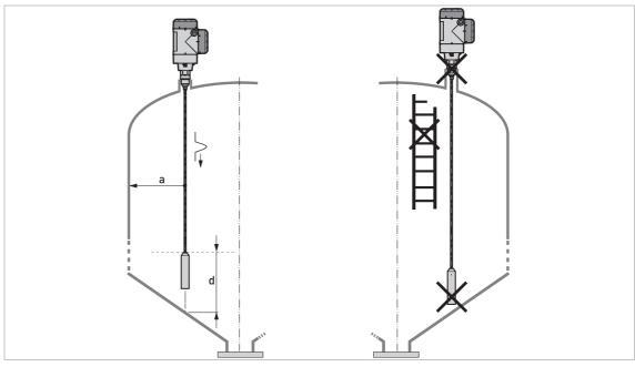
Figure 3-20: Installation recommendations for solids a  $\geq$  300 mm / 12" d  $\geq$  300 mm / 12"
