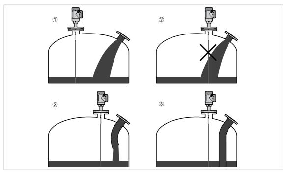
Figure 3-5: Do not put the device near to a product inlet
