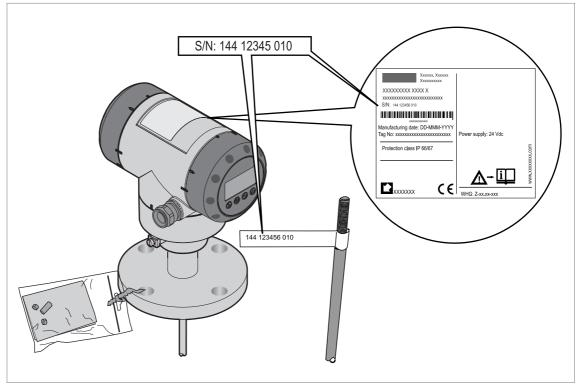
Figure 3-23: Check the order number on each component
