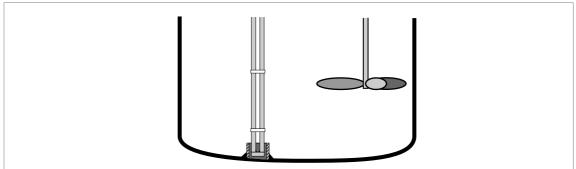
Figure 3-12: How to attach a double rod probe to keep it straight
