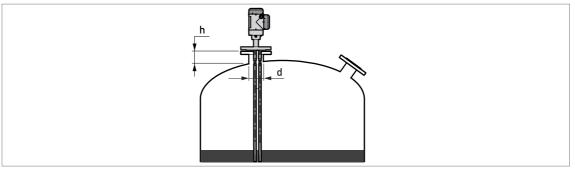
Figure 3-9: Recommended nozzle dimensions for double rod and double cable probes  $d\geq 50$  mm / 2°, where d is the diameter of the tank nozzle
