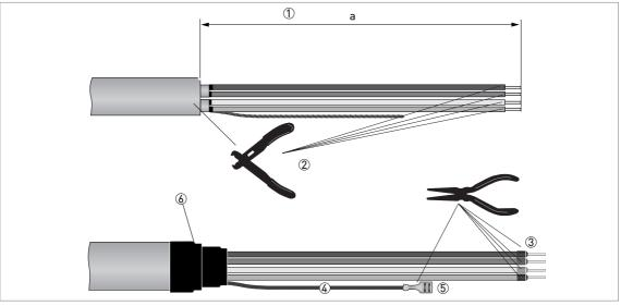
Figure 4-7: How to prepare the signal cable
