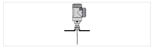
Figure 3-34: Threaded connection
