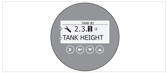
Figure 5-2: Local display screen layout in configuration mode
