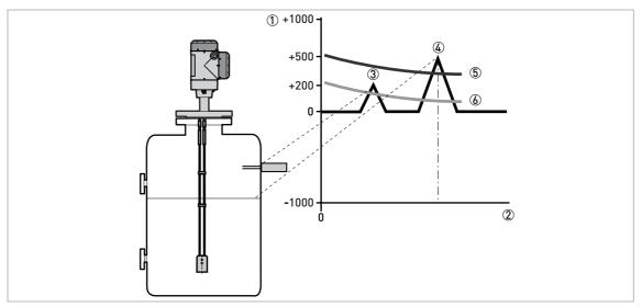
Figure 6-7: Signal intensity/distance graph: thresholds
