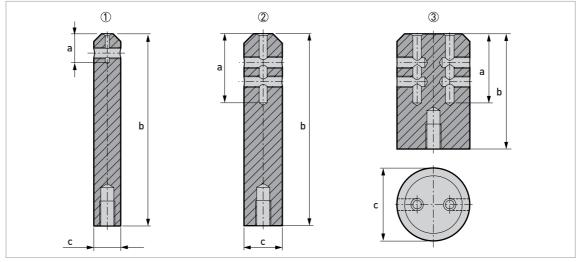
Figure 6-8: Dimensions of the counterweights
