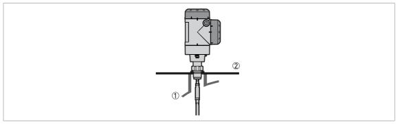
Figure 3-37: Installation in a non-metallic tank or pit with a thread connection
