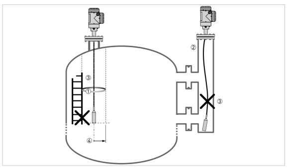
Figure 3-11: Installation recommendations for liquids
