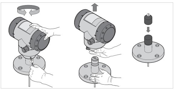
Figure 3-39: How to turn or remove the signal converter
