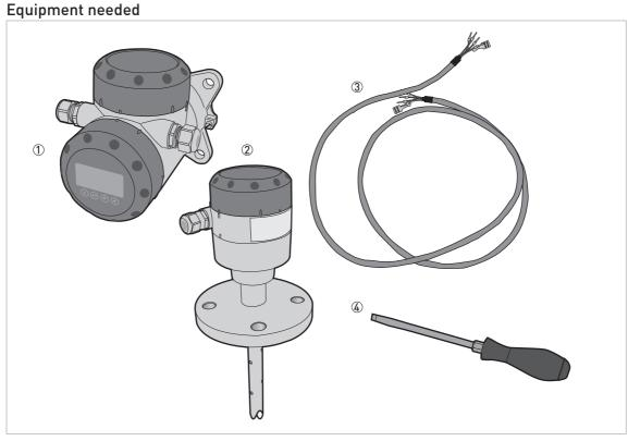
Figure 4-8: Equipment needed to prepare the signal cable
