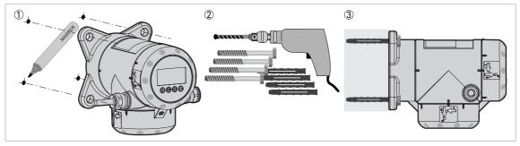
Figure 3-38: Wall support for the remote version (attached to the remote converter)
