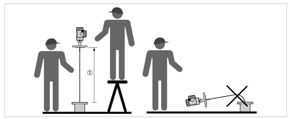
Figure 3-36: Installation of devices with cable probes (1) >1 m / 3½ ft
