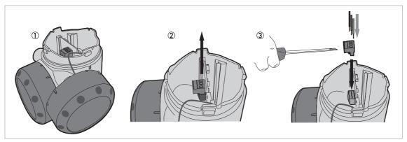
Figure 4-3: Procedure for electrical installation
