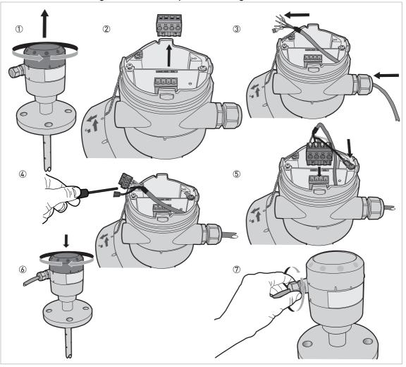
How to connect the signal cable to the probe housing
