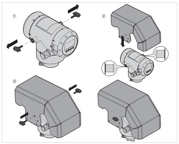
Figure 3-41: Installation of the weather protection (general procedure)
