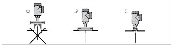
Figure 3-6: How to prevent build up of product around the process connection
