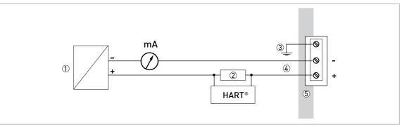
Figure 4-12: Electrical connections for non-Ex devices
