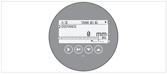
Figure 5-1: Local display screen layout in Normal mode
