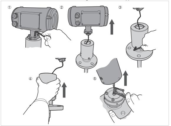
Procedure 2B: How to remove the BM 100 signal converter (Ex-approved devices)
