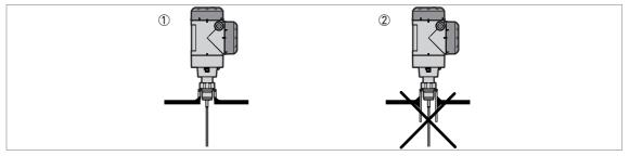
Figure 3-8: Sockets for threaded process connections
