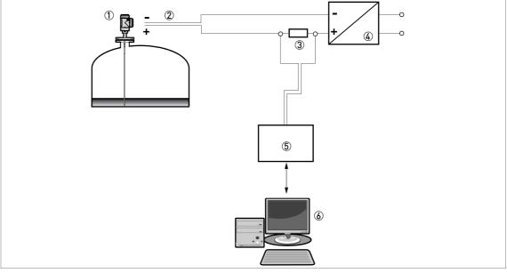
Figure 4-14: Point-to-point connection (non-Ex)
