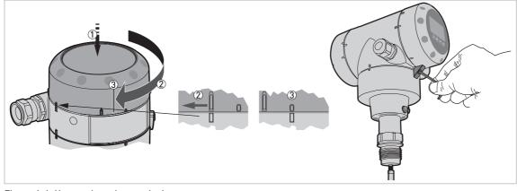
Figure 4-4: How to close the terminal compartment cover
