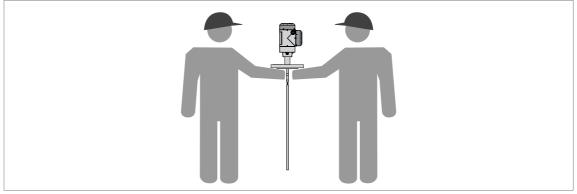
Figure 3-2: How to hold the device
