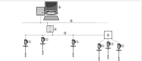
Figure 4-16: FOUNDATION™ fieldbus network (non-Ex)
