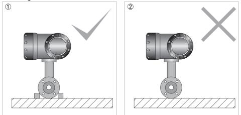
1 When standing the meter prior to installation, use blocks or similar to keep the meter upright. 2 NEVER stand the meter upright without blocks (or similar) .
