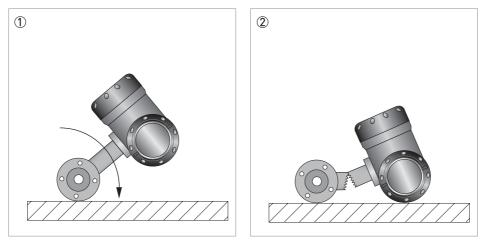
1 If the meter is not blocked it can roll over
