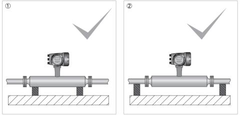
① The meter can be supported directly by its body
