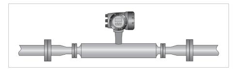
Always avoid extreme step changes in pipe size. Use pipework reducers, where there is a large difference between pipework size and meter flanges.
