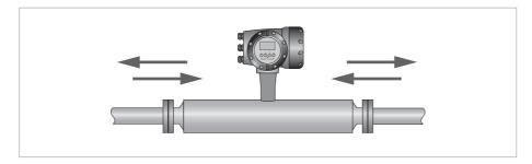
Mass flowmeters have a maximum level of force (negative or positive) that can be applied to the ends of the meter. Refer to the table below for permitted forces.
