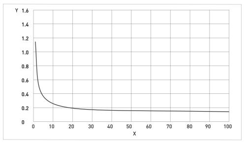
X flow rate [%] Y measuring error [%]
