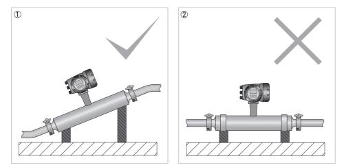
Install the meter at an angle to allow self-draining.
