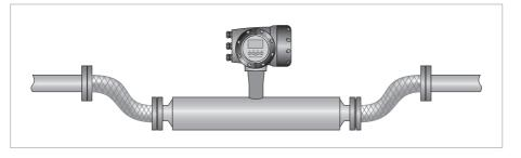
Flexible connections can be used but because of the high flow rates associated with large diameter meters, it is recommended that flexible connections are not used on meters larger than size 80.
