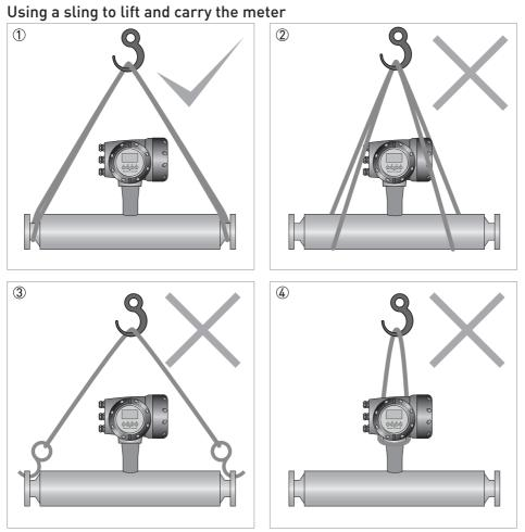
Use a well maintained sling to lift the meter by the spigots.
