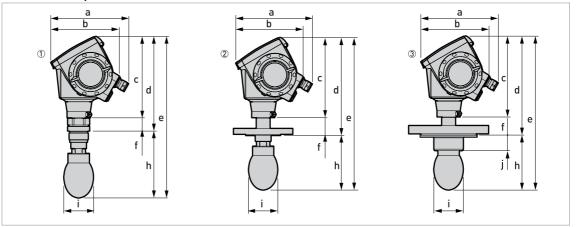
Figure 8-14: DN80/3" Drop antenna versions
