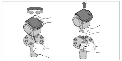
**Figure 3-23: How to turn or remove the signal converter** Tool: 5 mm Allen wrench
