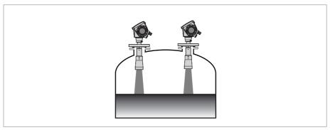
Figure 3-6: More than 1 FMCW radar level meter can be operated in a tank
