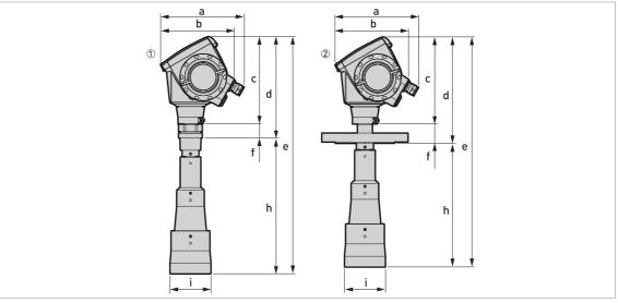
Figure 8-13: DN100/4" horn antenna versions
