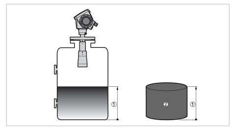
Figure 9-2: Measurement definitions: level
