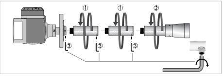
Figure 3-21: Horn antenna - how to attach antenna extensions
