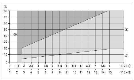
Figure 8-2: Selection of antenna for liquid applications (graph of distance in m against  $\epsilon_r$ )
