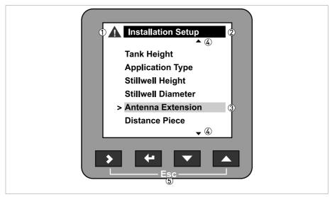
Figure 5-1: Local display screen layout
