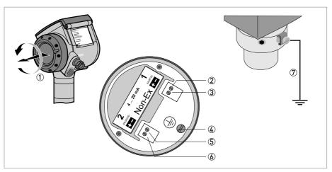
Figure 4-1: Electrical installation
