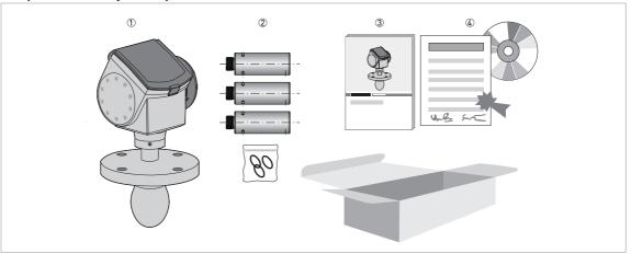
Figure 2-2: Scope of delivery - Drop antenna
