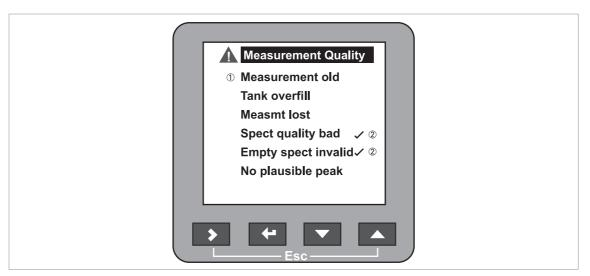
Figure 6-11: Measurement quality in supervisor mode
