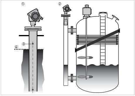
Figure 3-9: Installation recommendations for standpipes (stilling wells and bypass chambers)
