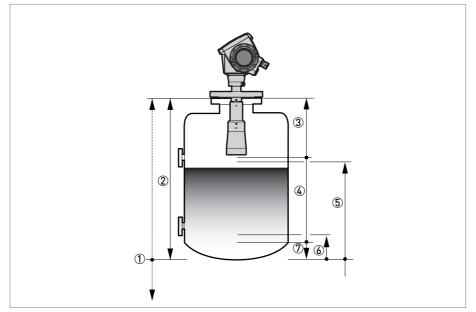
Figure 6-6: Level measurement
