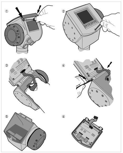
Figure 7-1: Removal of the device display cover
