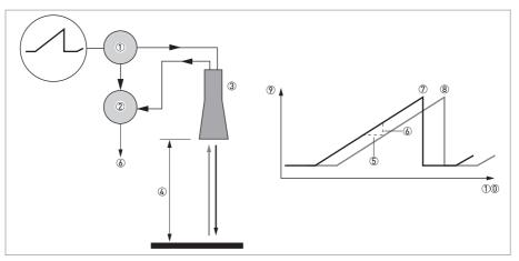
Figure 8-1: Measuring principle of FMCW radar
