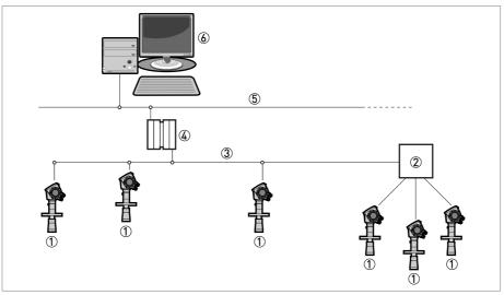
Figure 4-6: FOUNDATION Fieldbus™ network (non-Ex)
