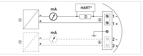
Figure 4-2: Electrical connections for non-Ex devices
