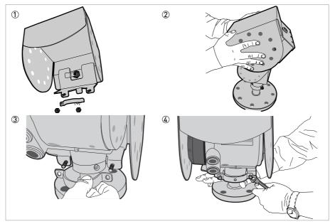
Figure 3-24: Installation of the weather protection
