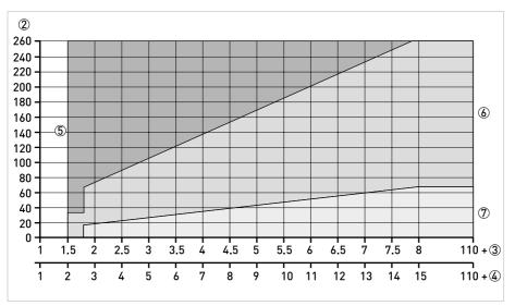
Figure 8-3: Selection of antenna for liquid applications (graph of distance in ft against  $\varepsilon_r$ )
