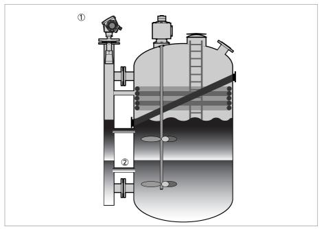
Figure 3-12: Installation recommendations for bypass chambers that contain more than one liquid ① Bypass chamber
