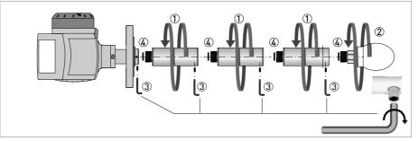
Figure 3-22: Drop antenna - how to attach antenna extensions
