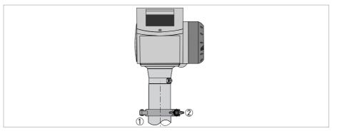
Figure 3-18: Tri-Clamp $^{\ensuremath{\mathbb{R}}}$  connection
