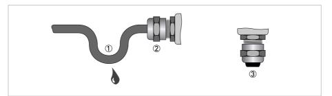
Figure 4-3: How to make the installation agree with protection category IP 67
