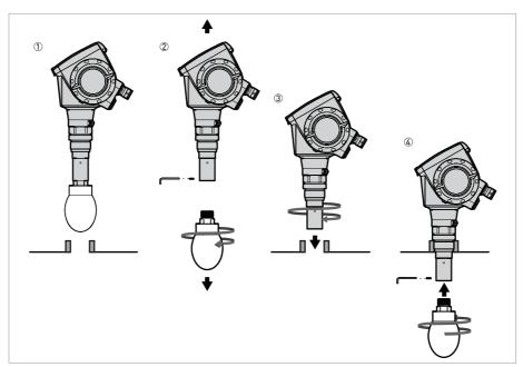
Figure 3-16: How to attach the device if the antenna is smaller than the process connection
