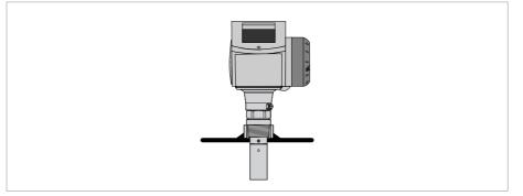
Figure 3-15: Threaded connection
