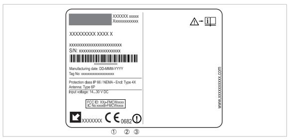
Figure 1-1: Radio approval information on the nameplate
