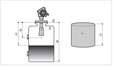
Figure 9-1: Measurement definitions: distance
