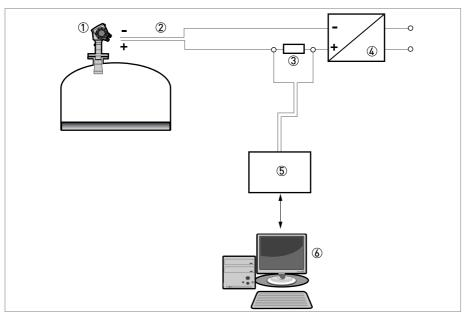
Figure 4-4: Point-to-point connection (non-Ex)
