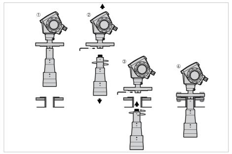
Figure 3-14: How to attach the device if the antenna is smaller than the process connection
