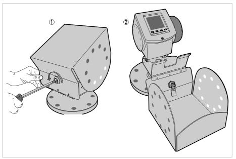
Figure 3-25: How to open the weather protection
