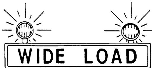
This sign is designed to be mounted on a vehicle top, carriers or an equivalent surface. It has 2 positions: upright when in use and folded flat on the carrier when not in use.
