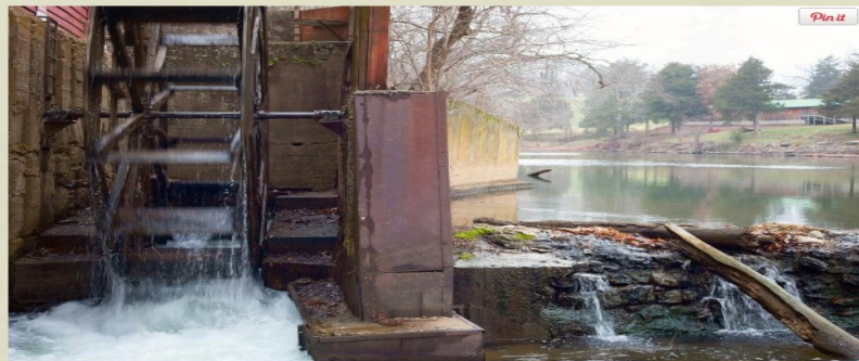
War Eagle Mill's 18-foot undershot water wheel rotates when water strikes the paddles or blades at the bottom of the wheel. The force of the water's movement drives the blades of the wheel, which rotates a turbine that drives the mill's machinery. This, in turn, allows the millstone to grind grain into flour.
