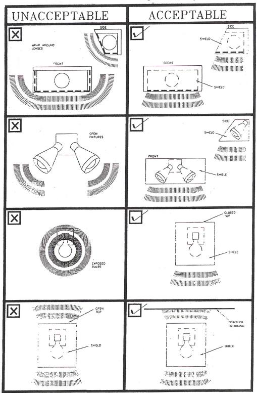
The angle of light deflection from hoods or shields is to be no more than 45 degrees perpendicular through the light source (bulb or tube).
