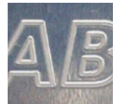
VIBRATING DOT PEEN Characters are marked with a small pin while vibrating. Highly recommended for fast marking with very high quality needs.
