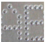
CONTROLLED DOT PEEN Font characters are created with possibility to specify the density of the dots to be marked from 0 to 80 pixels/cm. Recommended for deep marking.
