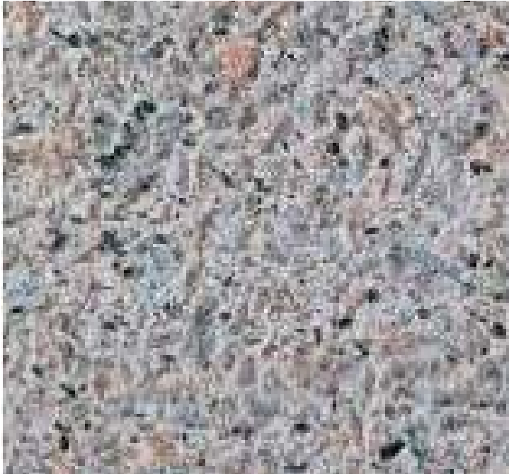
BASE BUILDING: PRECAST PANEL Gate Precast: Color 152 Sandblasted white w/ granite aggregate.
