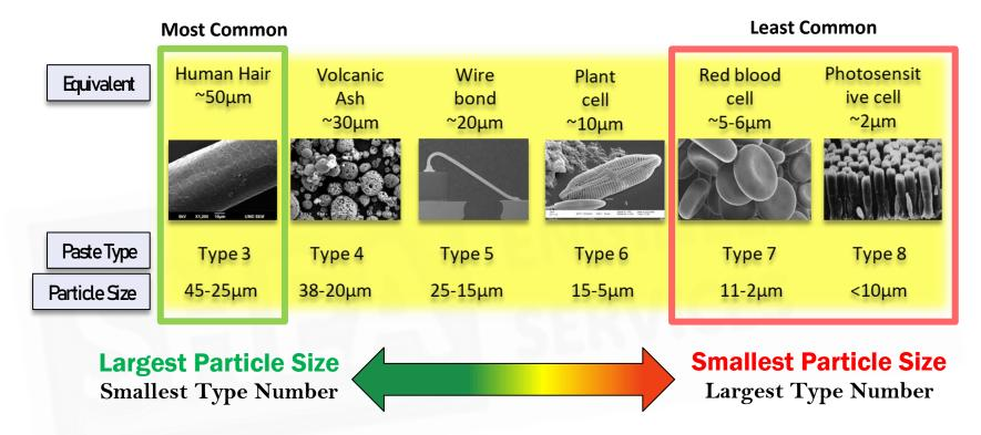
Smaller particles have higher oxide-to-solder ratios which make them more difficult to reflow.
