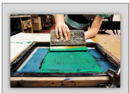
A blade is pulled across the surface, pressing the print media through the stencil on the surface.
