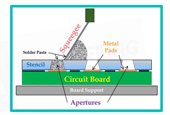
The goal of printing is to deposit the proper <u>amount</u> of solder paste at the proper <u>location</u> in the proper <u>shape</u>.
