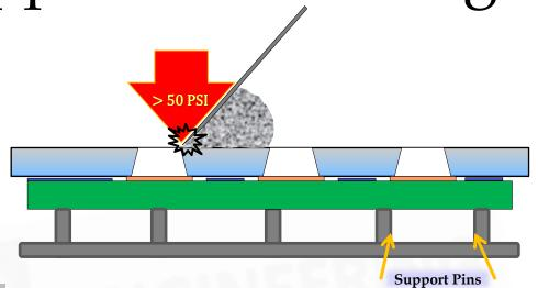
Without *proper* **Cond Support** the pressure of the squeegee causes the stencil and board to deflect and snapback at different rates, smearing the print.
