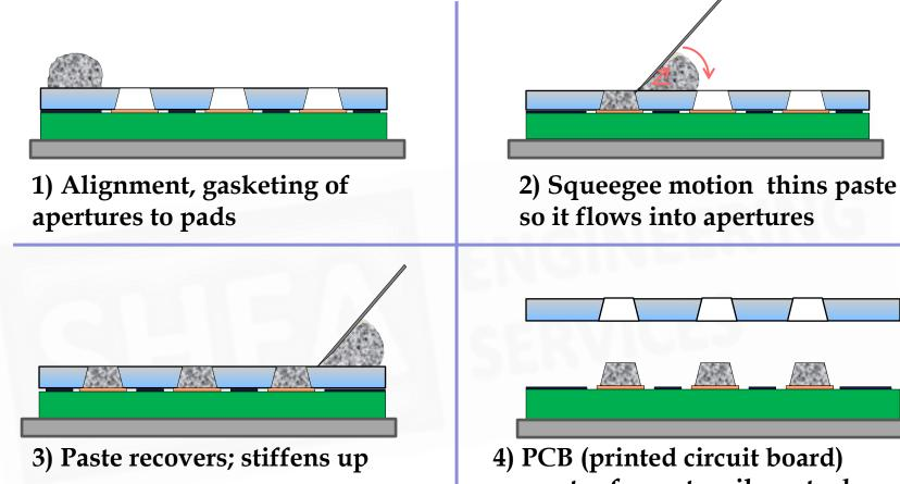
separates from stencil; paste deposits release from stencil onto pads
