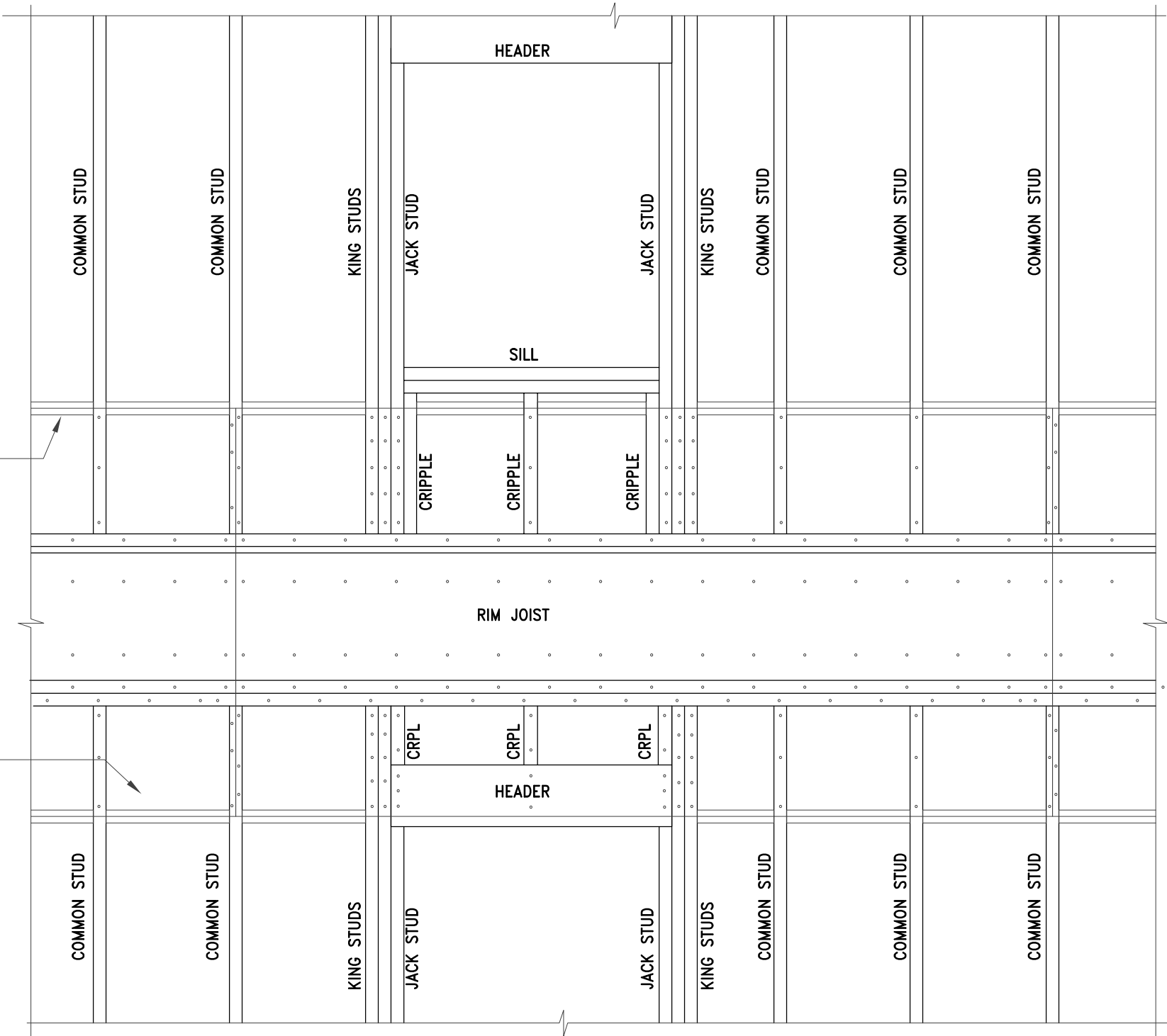
1 PLYWOOD TIE PANEL DETAIL ACROSS FLOOR LEVELS SCALE: 3/4"=1'-0"
