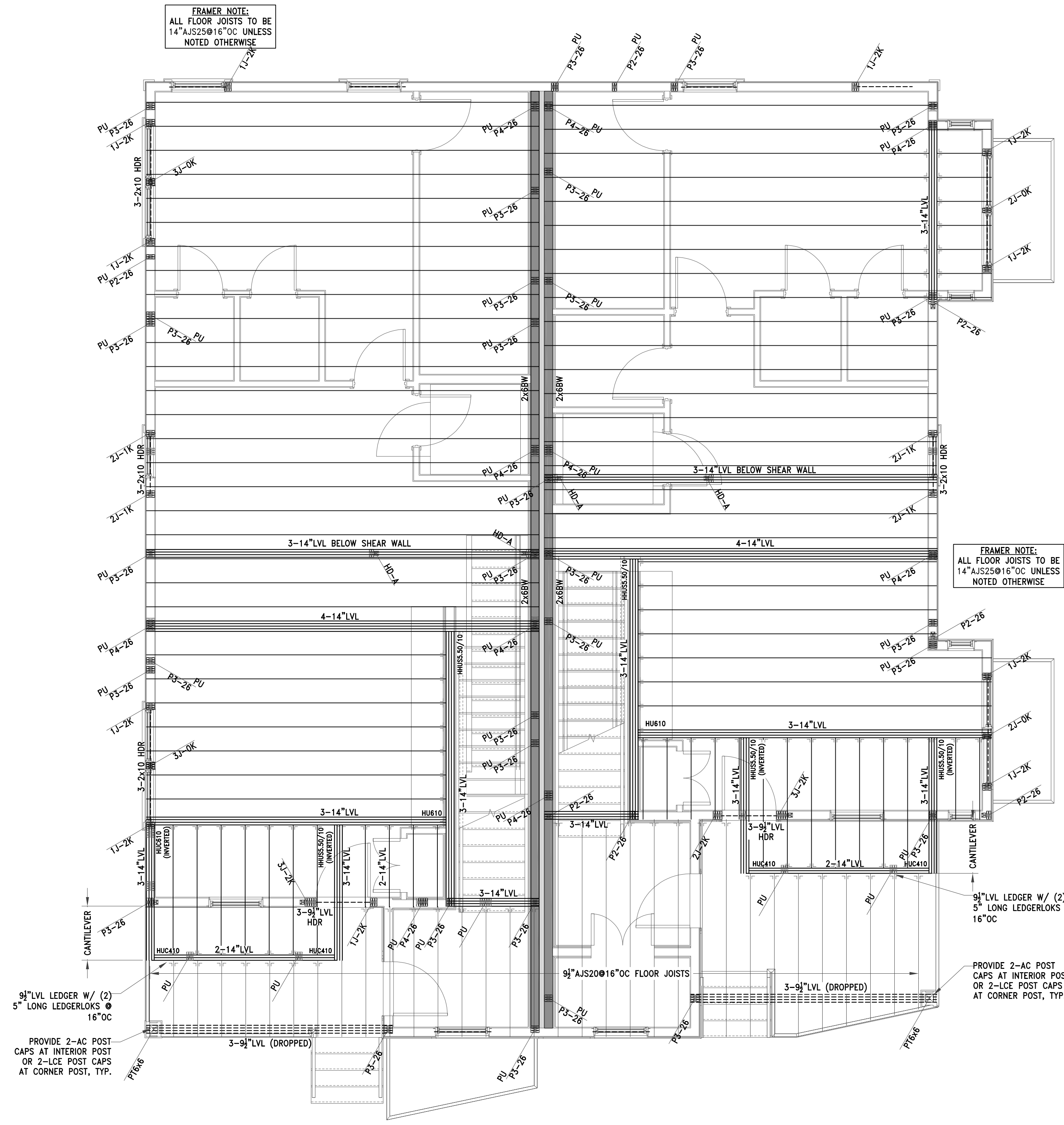
SECOND FLOOR FRAMING SCALE: 1/4"=1'-0"
