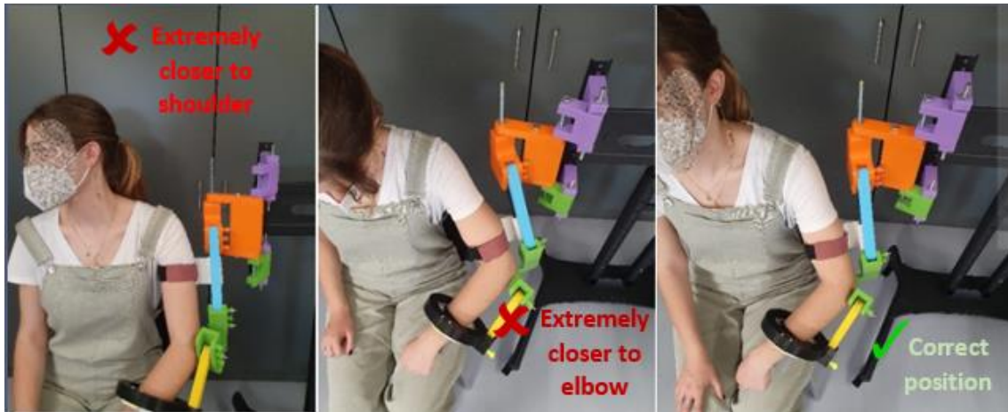
Figure 65: Wrong and correct position of Velcros for attaching upper arm support
