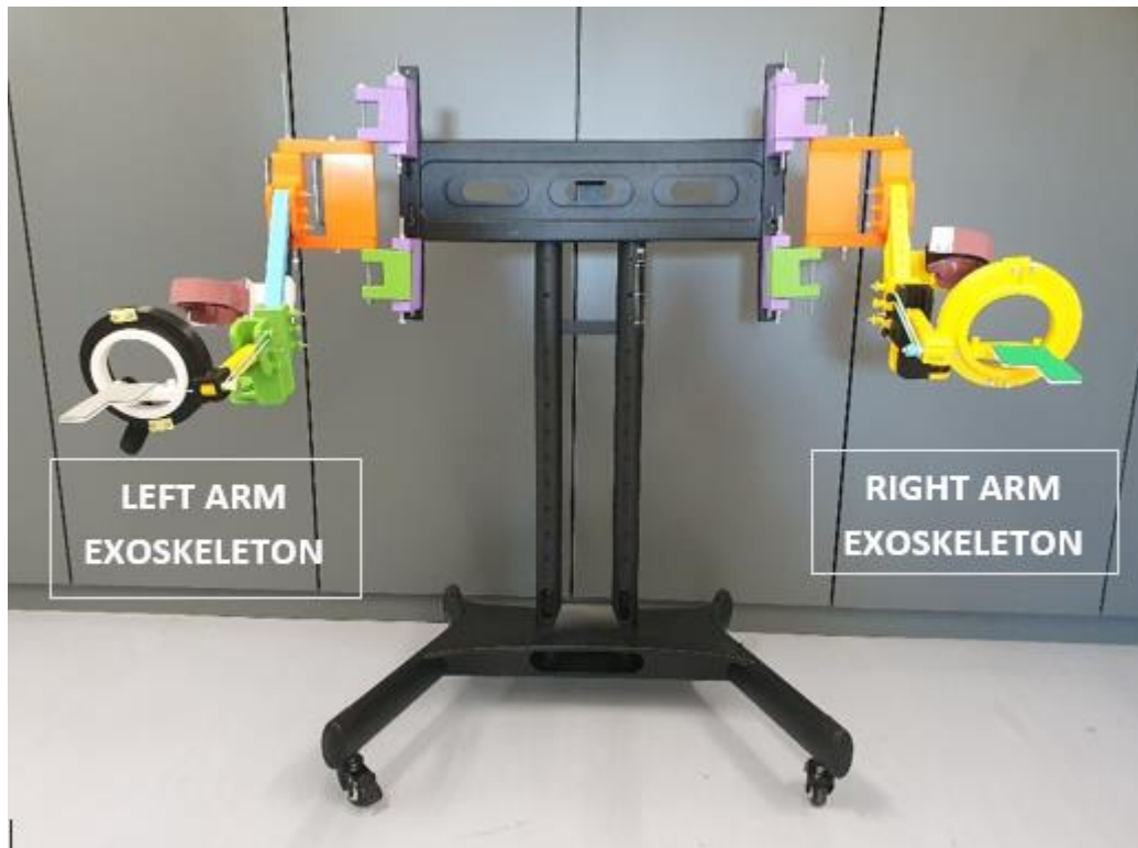
Figure 52: Right and left exoskeletons assembled in current support platform
