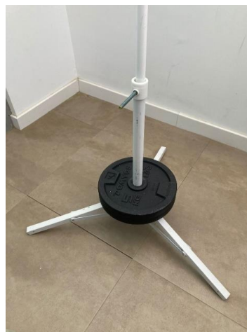
Figure 44: First support platform made with umbrella tripod, weights and threaded rod
