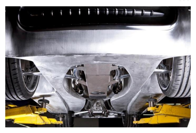
The suspension is inspired by F1 and Indy car designs but utilizes only one spring mounted horizontally. The front suspension has an A-arm on top that connects to the nose cone, an H-arm that connects to the reinforced oil pan, pushrods, and a sway bar that is two pieces and coupled in the middle.
