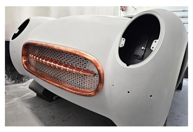
Like the body panels, all the trim and various bits are one-off parts either handmade or created using CNC machines or 3D printing.
