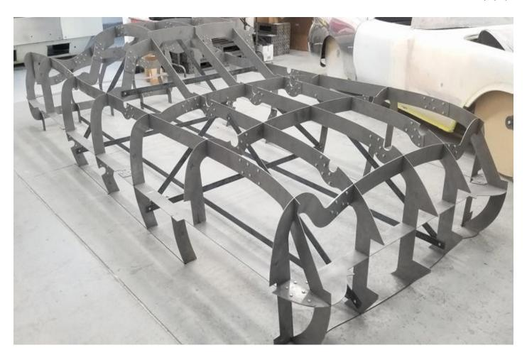
There was a time when the best cars on the planet were formed by hand, and that was the case here. The build crew used a buck to get the shape of the aluminum sheetmetal.
