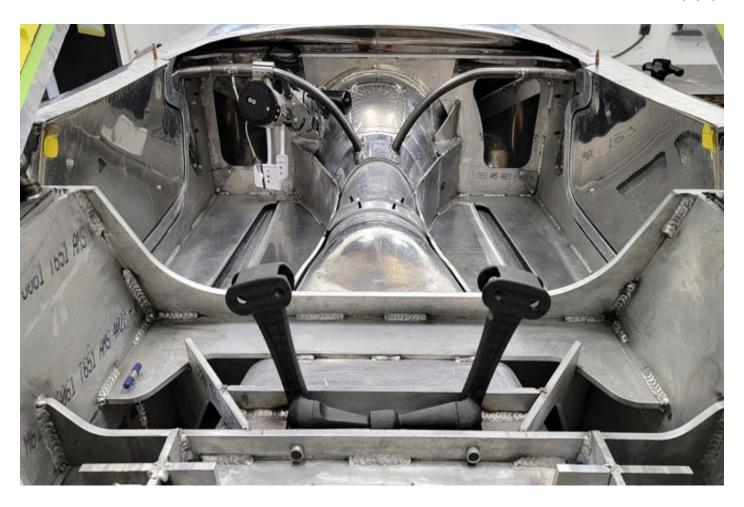
A modified automatic <u>C7</u> Corvette transaxle was used. The torque tube was extended, and the housing was replaced with one that was thicker and more structurally sound. Race Cast Engineering also cast a piece Kindig designed and calls the nose cone. It is attached to the front of the engine and houses the rack-and-pinion steering, the pass-through for the engine cooling, and some suspension components like the sway bar and front spring.
