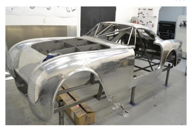
The top and outer shell were hand-formed out of 3003 aluminum. We can only imagine the hundreds of hours spent shaping the panels to conform to the buck.
