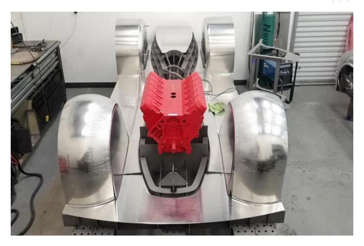
The floor and bottom were built using a reinforced structure of thicker 6061 sheetmetal that was sandwiched together to create a monocoque/unibody. Look closely at that mockup <u>LS engine</u> and count the cylinders—we'll get to that in a bit.
