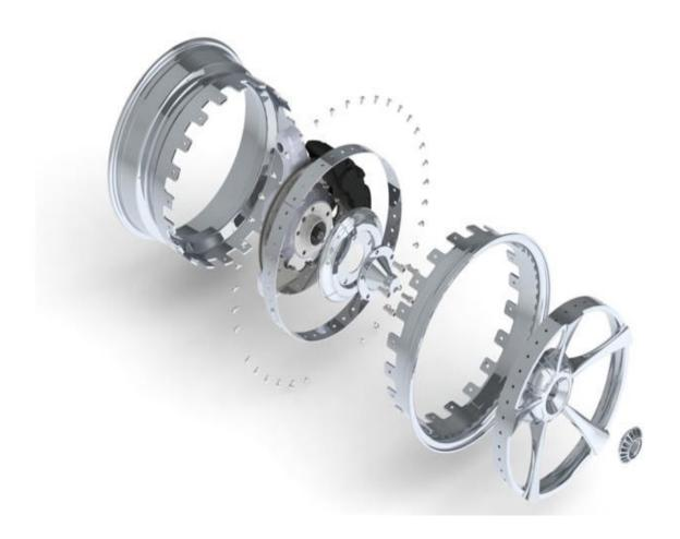
Dave Kindig came up with this proprietary design for the wheels, where all the hardware is hidden. His design was sent to EVOD, which machined the 19x8-inch front and 20x12-inch rear monolug five-spoke billet wheels. When vendors are used for a Ridler build, they know how important secrecy is to the project.
