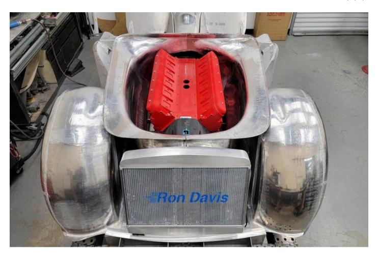
Everything about the car is unique, and although this had to be a working and driving car, Kindig wanted to avoid the clutter of the parts needed to make that happen. The drivetrain is bolted to that inner structure, making it an integral part of the car's load-bearing surface, and as many components as possible were hidden from view.
