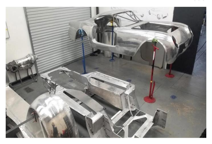
The car was built in three main pieces: the top/outer sheets, the floor/bottom, and the doors and hood. No donor car was used, and the whole car was designed and built from scratch, in-house.
