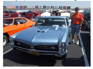
In 2010 this 225K mile GTO received a full rotisserie restoration, but with a few modifications for drivability and comfort. For starters, it has a 5 speed Tremec trans., 4 wheel disk brakes, 15" honeycomb wheels, vintage air A/C and Global West full suspension. This '67 GTO has all the handling and stopping power plus creature comforts of a newer GTO.
