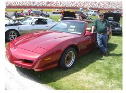
Dave bought this car new @ Dick Keffer Pontiac in Charlotte and it has the 5.0 Liter EFI engine and Automatic transmission with optional Aero Package, which includes the front air dam and ground affects.
