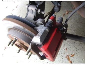
First remove the caliper bolts. Seen in picture below - loosened.
