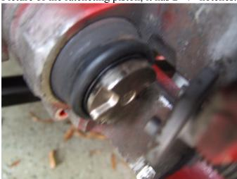
I borrowed a MAC Tool to screw the piston back in.
