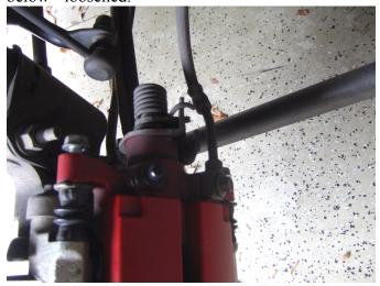
Then remove the caliper holding bracket if you are replacing the rotor. These have locktight on them, so you really need some force to loosen them.
