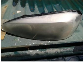
I first wet sanded the whole headlight (about 15-20 min.) on each headlight to remove all the crusty baked on clear coat, and then finished with the grey scotch bright pad. I then wiped them off with water with a little bit of liquid dawn detergent.
