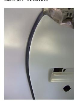
I made a shim out of sheet metal that fit perfectly in the space to fill the gap and then welded it in place (the holes in the middle were for weld penetration).
