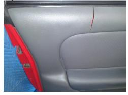
Subject: 1999 Trans Am – Driver's and passenger's door panels both cracked all the way through.
