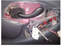
First remove the small screw from the door handle escheon, then remove the large phillip's shown in the picture and 2 other large phillip's below, then pop out the window switch and disconnect wires.
