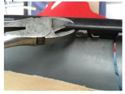
Carefully remove 1 or 2 staples in front and behind the crack until you see the door panel relax. I just set the side cutters there, so you can see what tool I used and where!
