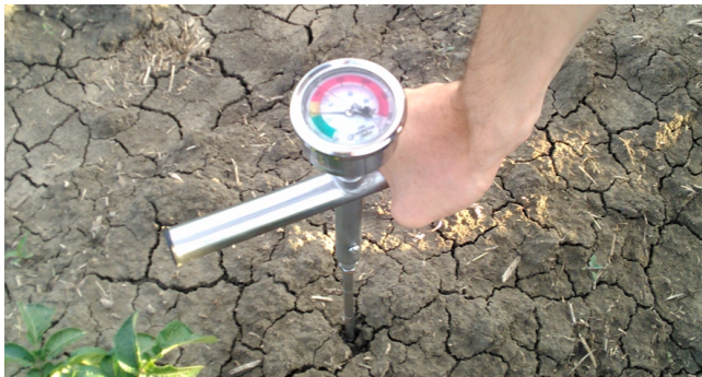
Penetrometer - measures the resistance to penetrate the soil
