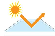
5400 windows are more energy efficient when ordered with optional Low E glass and an Argon gas-filled insulating glass unit. Low E glass helps keep homes warmer in winter and cooler in summer.
