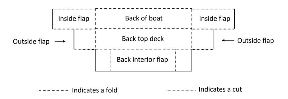
Starting at the top, the first fold brings the back into a vertical position. The two side flaps are moved to the inside, parallel to the sides. The next fold is toward the front of the boat and creates the back deck. The outside flaps are bent down toward the bottom of the boat. The two short pieces lay on the top of the sides and the interior flap is bent down, into the sitting area of the boat.
