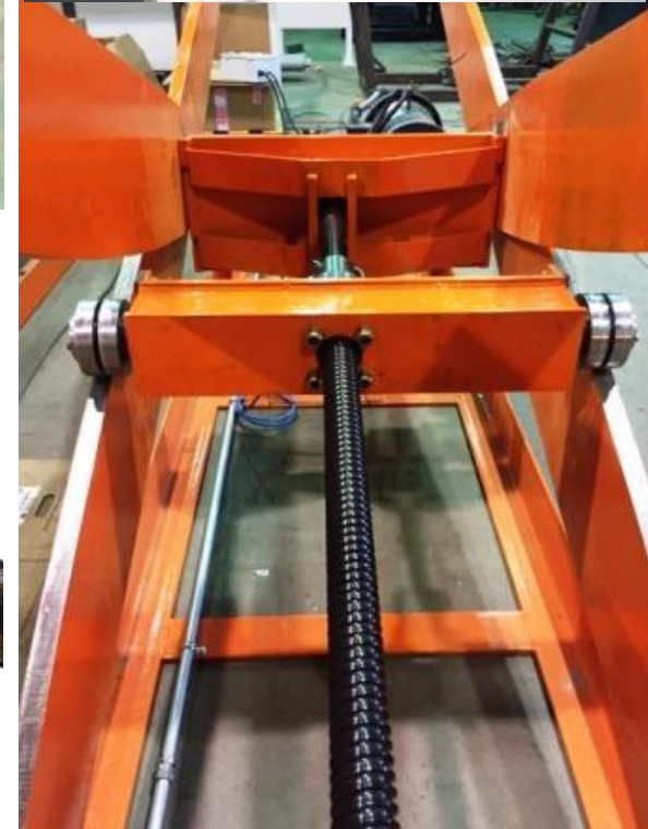
LEAD SCREW ARRANGEMENT ON ELECTRIC SCISSOR LIFT
