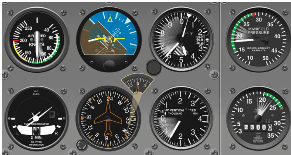
Figure 1-3: Instrument Indications in a Spiral Dive, FAA Instrument Flying Handbook
