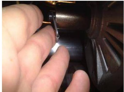
Remove the control handle with a 3/32 Allen wrench
