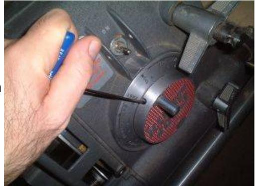
Remove the three large screws. (They are numbered in the photo.)
