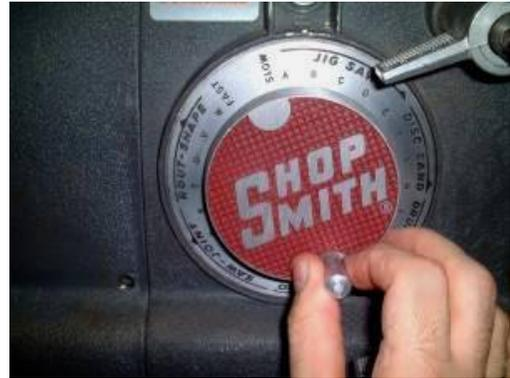
Use a small screwdriver to hold the set screw, then loosen the jam nut.
