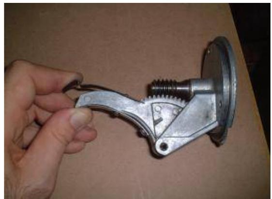
This is a shot from inside of the Shopsmith. This is the retaining-loop. Normally, it is hooked over the leaf spring that you saw in the last photo. Once the leaf spring is depressed, you sort of roll the retaining-loop off of the leaf spring. It's not the easiest thing in the world, but, with a little patience, it can be done.
