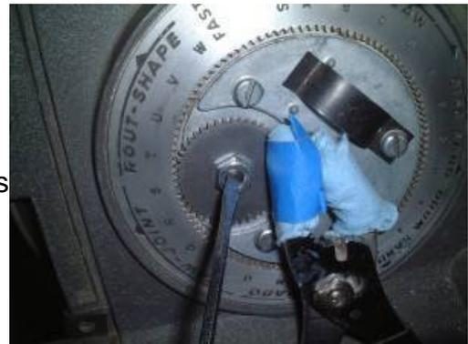
Turn off your Shopsmith. Re-tighten the jam nut. Press in and turn the speed dial until it reads "fast."
