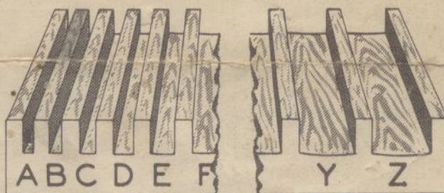
gauge stick showing graduated notches in alphabetical sequence
