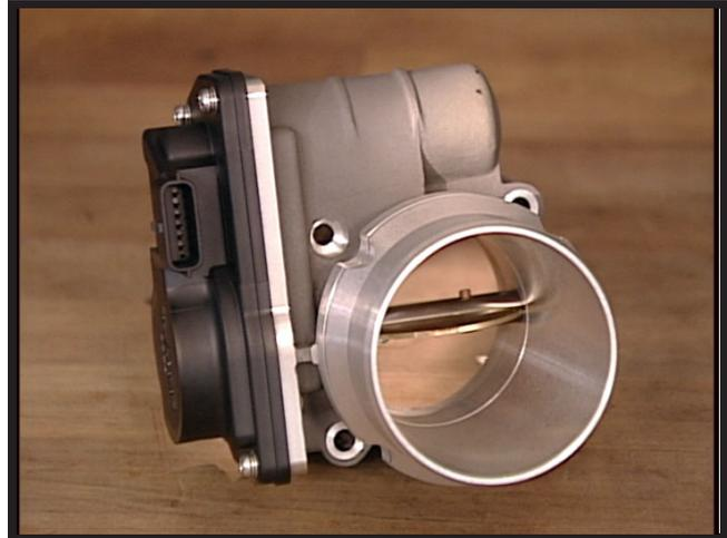
**Figure 4-5, Air Intake Valve**
