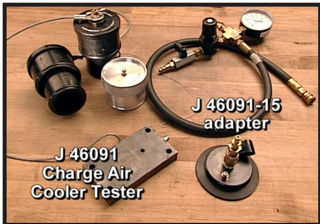
**Figure 7-2, Charge Air Cooler Tester and Adapter**
