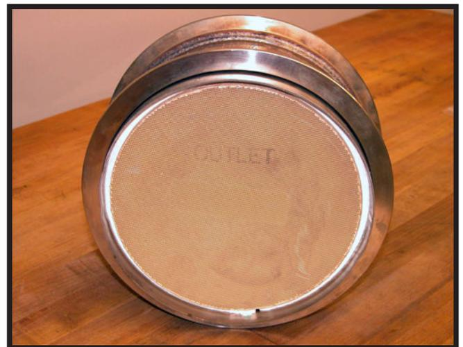
**Figure 5-2, Diesel Oxidation Catalyst (DOC)**
