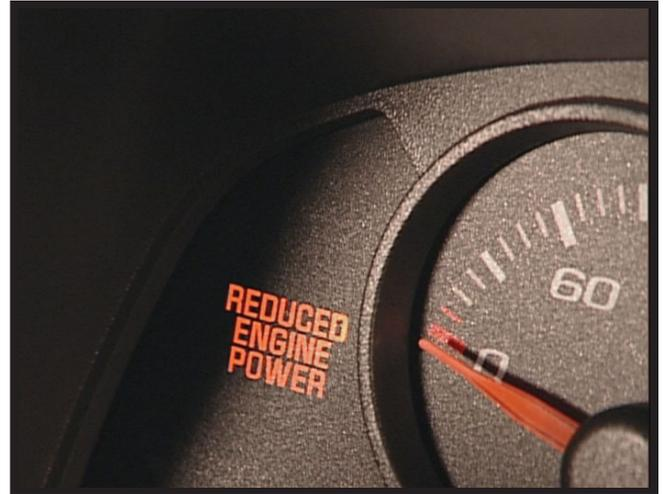
**Figure 7-1, "Reduced Engine Power" Lamp for Limp Home Mode**
