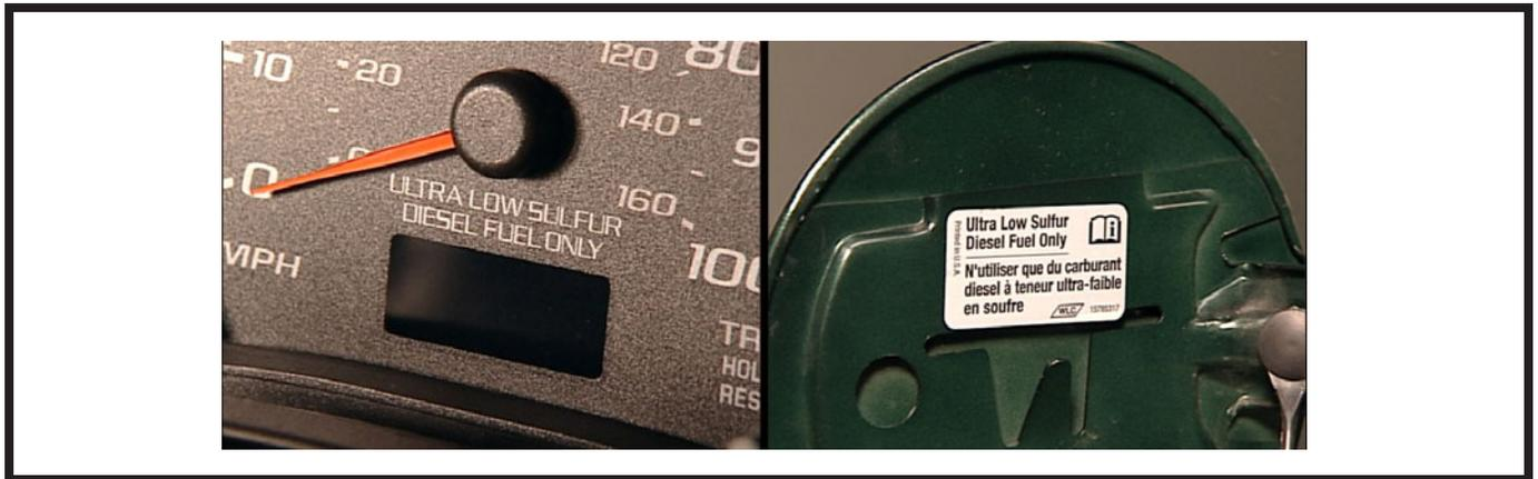
Figure 3-4, Vehicle Fuel Labels
