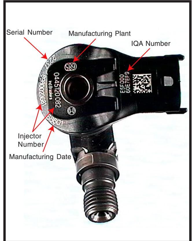
Figure 4-3, Duramax LMM Fuel Injector
