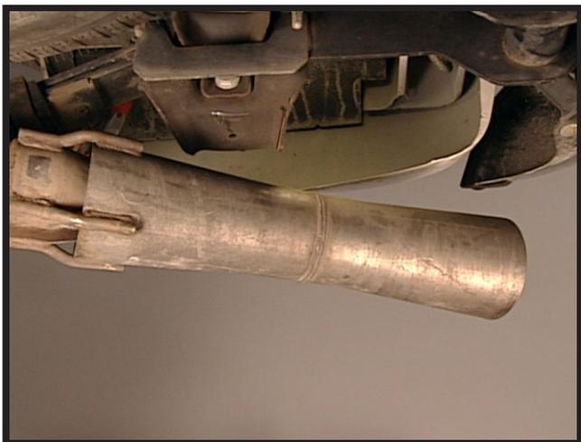
**Figure 5-8, Tailpipe Exhaust Air Cooler Silverado/Sierra**
