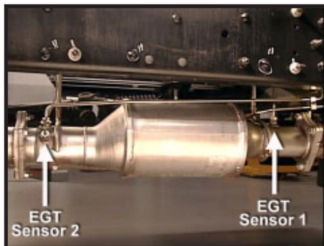
**Figure 5-6, EGT Sensor 1 and EGT Sensor 2 (Medium Duty)**
