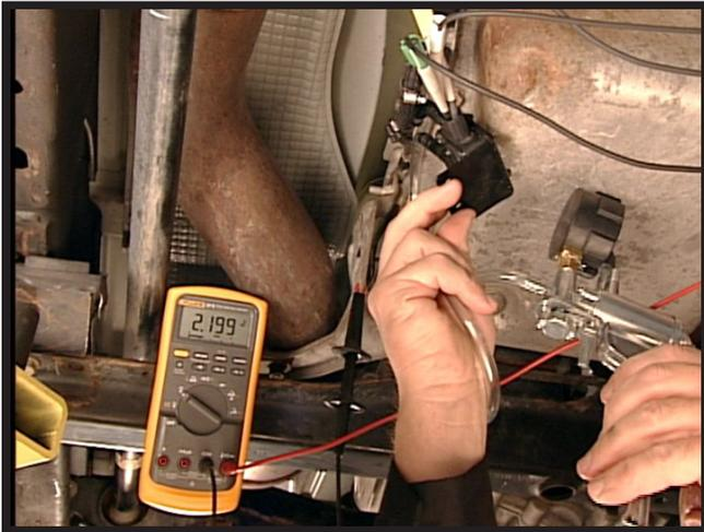
**Figure 7-4, Testing DPS with Mity Vac**
