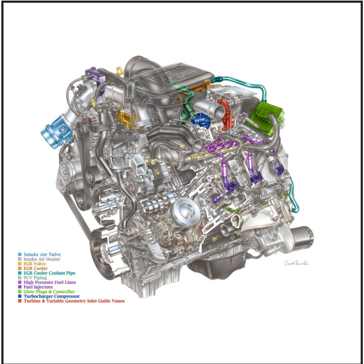
Figure 4-1, Duramax Diesel 6600, RPO LMM
