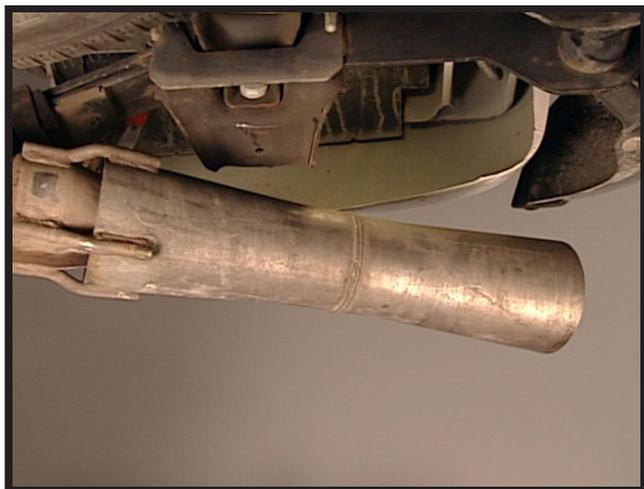
**Figure 5-8, Tailpipe Exhaust Air Cooler Silverado/Sierra**
