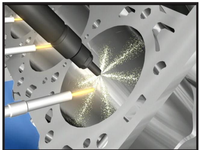
Figure 4-4, Injector Spray
