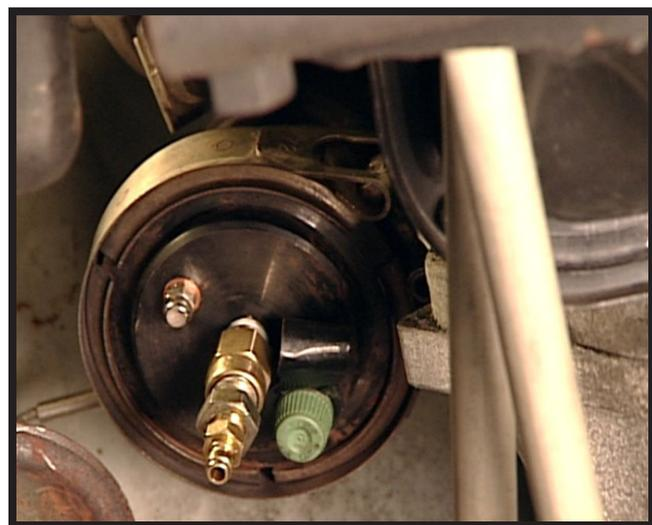
**Figure 7-3,** J 46091-15 Installed on Exhaust Downpipe
