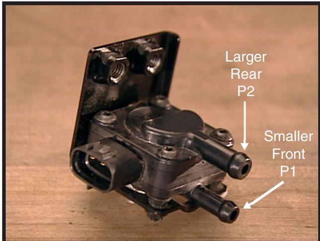
**Figure 5-7, Differential Pressure Sensor**
