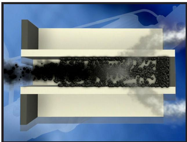
**Figure 5-4, DPF Channels Trap Particulate Matter**
