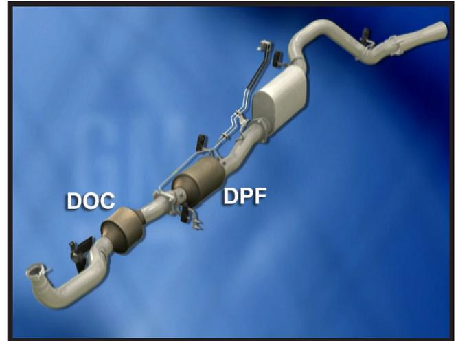
**Figure 5-1, Typical Duramax DPF System Configuration**
