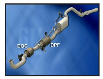
Figure 5-1, Typical Duramax DPF System Configuration
