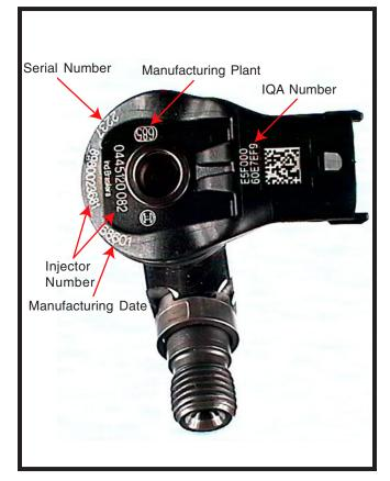
Figure 4-3, Duramax LMM Fuel Injector
