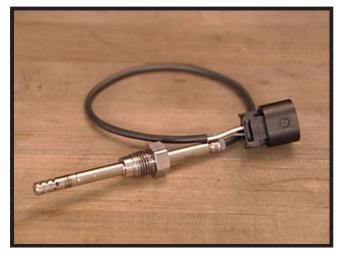
Figure 5-5, Exhaust Gas Temperature Sensor (EGT)
