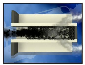
Figure 5-4, DPF Channels Trap Particulate Matter
