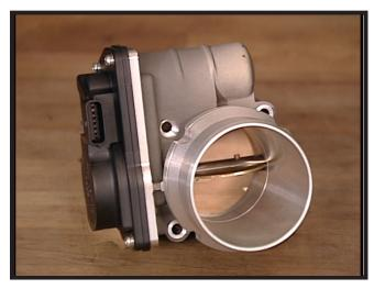
Figure 4-5, Air Intake Valve
