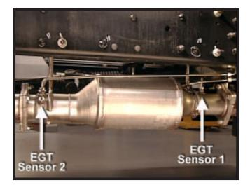
Figure 5-6, EGT Sensor 1 and EGT Sensor 2 (Medium Duty)
