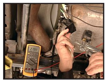
Figure 7-4, Testing DPS with Mity Vac
