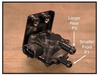
Figure 5-7, Differential Pressure Sensor
