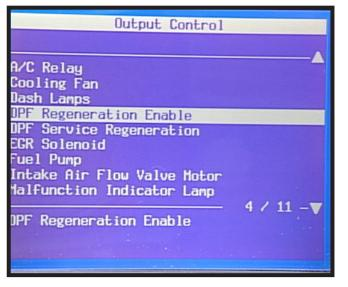
Figure 6-9, Scan Tool Regeneration Enable
