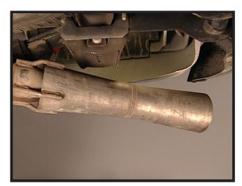
Figure 5-8, Tailpipe Exhaust Air Cooler Silverado/Sierra
